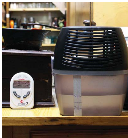
Figure 31: "Home" type dehumidifier and electronic thermo/hygrometer.
