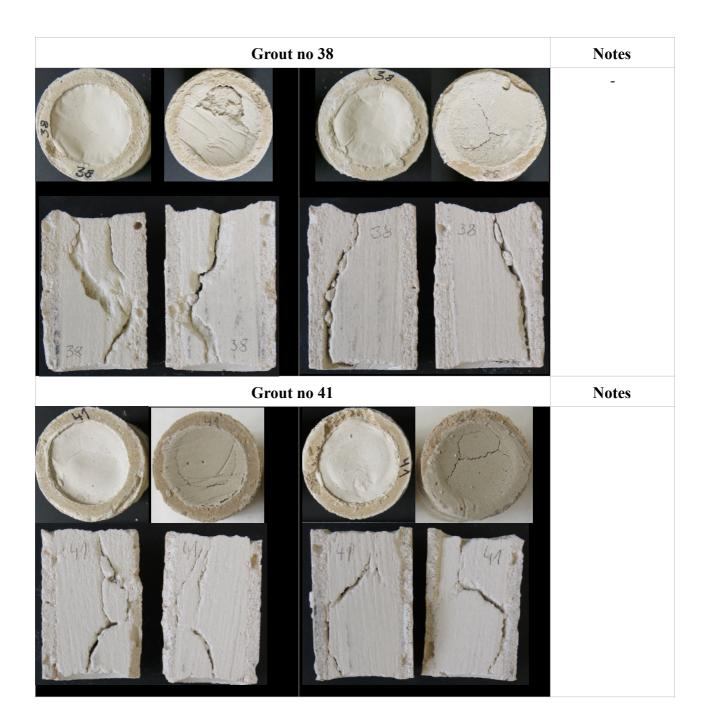
59. Shrinkage in cylinder test. Grouts with the evaluation mark number 4.
