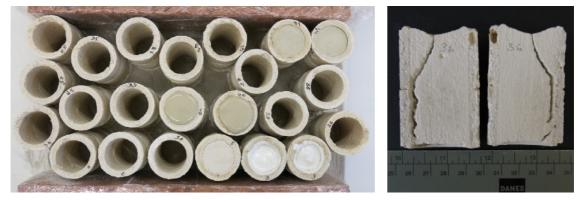
**38.** Casting the grouts inside the cylinders. The cured grout in the cylinder cut in halves.
