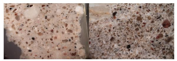
Fine particles of quartz (transparent/white) and granite (light red) sand can be seen in these optical microscope photographs, taken from the sand of both samples, TV-V-1 and TV-W-1 (see ill. 19 and 20).
