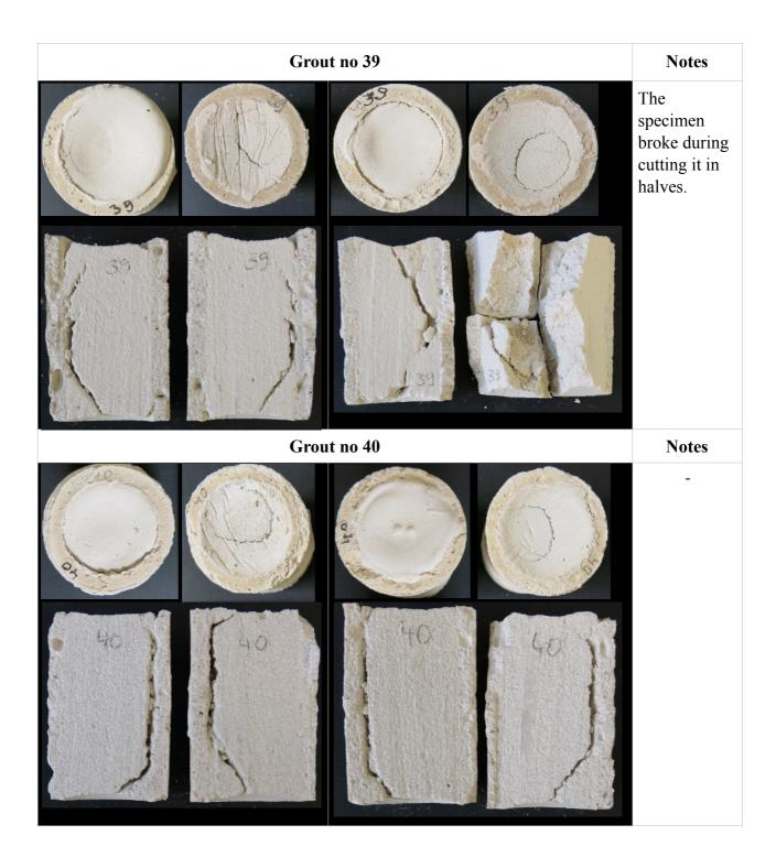
**58.** Shrinkage in cylinder test. Grouts with the evaluation mark number 3.
