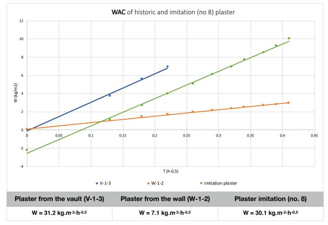
**15.** Water absorption coefficient of historic plasters from the vault (V-1-3), wall (W-1-2) and the plaster imitation number 8 (chosen to carry out laboratory testing of injection grouts).
