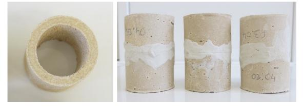
4. Two cylinders were used for each grout. After 21 days of curing, the specimens were cut in half to evaluate shrinkage (see ill. 38).
