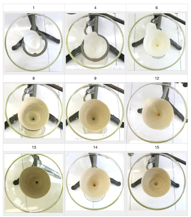
**49.** Grouts classified as **very fluid (evaluation mark: 0).** Each photo is marked with the grout number.
