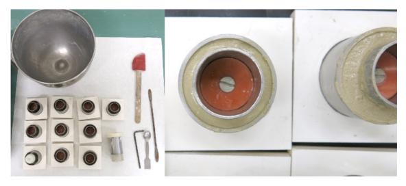
2. The inner surface of the specimen was coarsened before it was taken out of the cast, and left to cure for 28 days. The dimensions of the specimens were 40x40x5 mm (see ill. 36).
