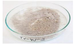
8. To calculate the percentage of the sand the total weight of the sand  $(2^{nd} \text{ weight})$  was subtracted from the weight of the crushed sample  $(1^{st} \text{ weight})$  and the result was multiplied with 100. The percentage of dissolved binder is equal with the percentage of the sand subtracted from the  $100\%.^{42}$
