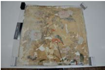
Figure 93. A small segment of a wallpaper was bleached with hydrogen peroxide. Before and after the treatment.
