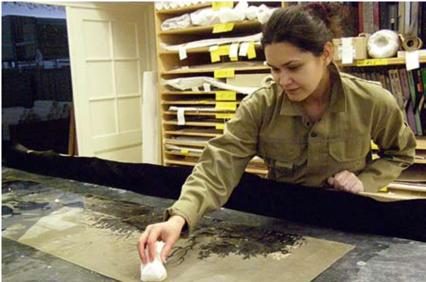
Figure 91. The impurities not absorbed by the blotters should be removed manually. Photo was taken during the relocation of the wallpaper collection of the German Wallpaper Museum in Kassel.
