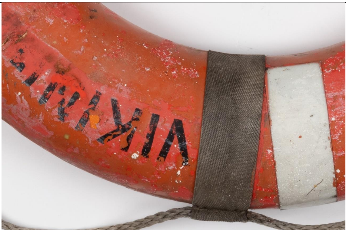
Photo 11 Flaking paint and its borders were stabilised to prevent future flaking. Authors: Anu Ansu & Berta Jänes, Estonian National Museum Date: 11.11.2024 Image size: 10 x 15 cm
